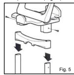
6. Slide the top brace down the legs until it reaches the top of the pressure washer. Secure the top brace to the pressure washer unit with the two (2) screws provided. (Fig. 6)
